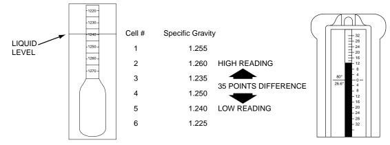
Figure 5. Reading a Battery Hydrometer
